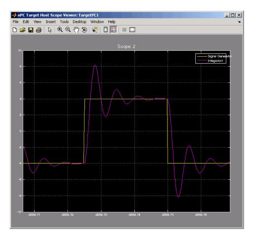
7 Add signals to the scope of type file. For example, to add signals Integrator1 and Signal Generator, right-click each signal and select Add to Scopes. From the Add to Scopes list, select Scope 3. (Note that you can also drag a signal from one scope to another to add that signal to another scope.)
