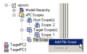
By default, xPC Target creates a file in the target PC C:\ directory. The name of the file typically consists of the scope object name, ScopeId, and the beginning letters of the first signal added to the scope.
