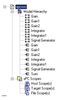
**4** To create a scope to display on the target PC, right-click the Target Scopes node under the xPC Scopes node.
