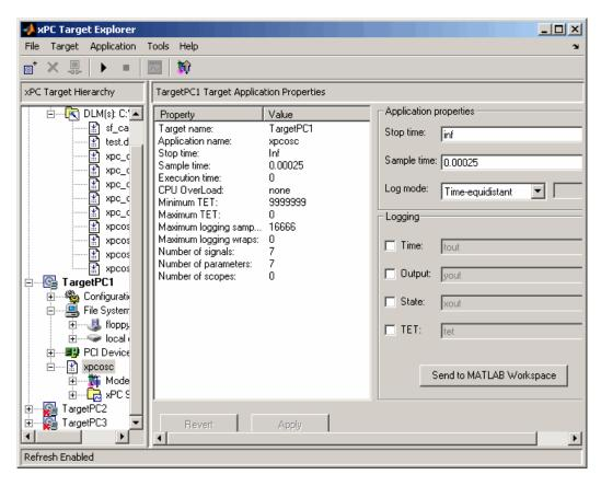
**3** To get the list of signals in the target application, expand the target application node, then expand the Model Hierarchy node under the target application node.
