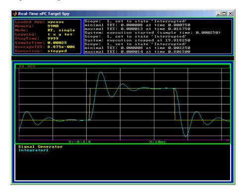
**4** Add signals to the host PC scope. For example, to add signals Integrator1 and Signal Generator, right-click each signal and select **Add to Scopes**. From the **Add to Scopes** list, select Scope 2. (Note that you can also drag a signal from one scope to another to add that signal to another scope.)
