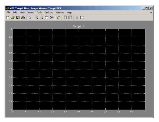
**10** To list the properties of the scope object Scope 2, click the xPC Target Explorer tab to return to that window, and left-click Scope 2. (Note that you can configure the docking view using the MATLAB docking feature.)
