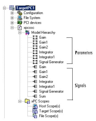
The Model Hierarchy expands to show the elements in the Simulink model.
