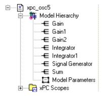
Note that the Model Hierarchy node displays a list of signals and an object called Model Parameters. Model Parameters contains the list of tunable inlined parameters.
