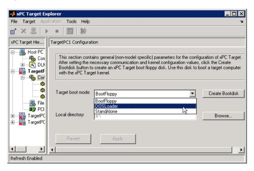
The default setting for the option **Target boot mode** is BootFloppy. When you are using BootFloppy, xPC Target must first create a target boot disk, which is then used to boot the target PC.
